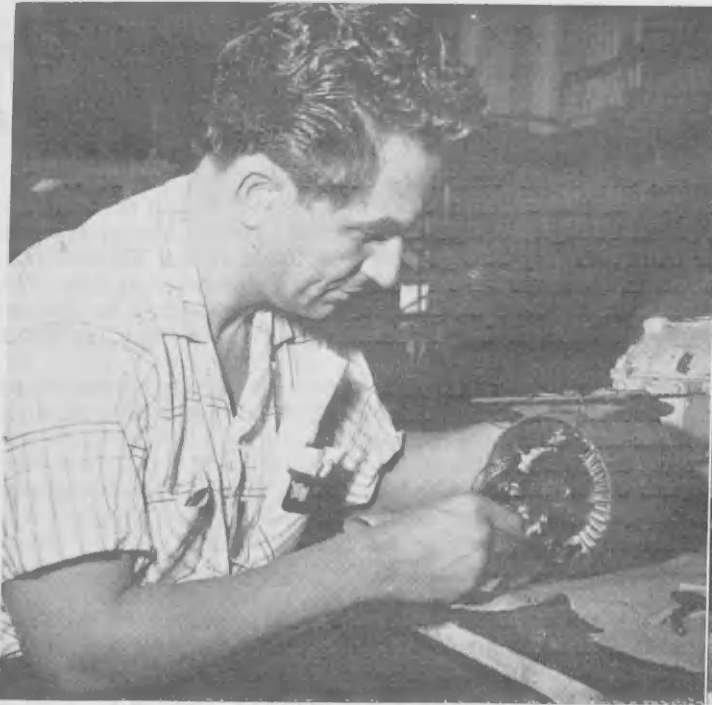
AN ELECTRICIAN, above, installs windings in a stator. Being hoisted, above right, is a squirrel cage rotor. Motors are integral parts of instrument controls, below.
